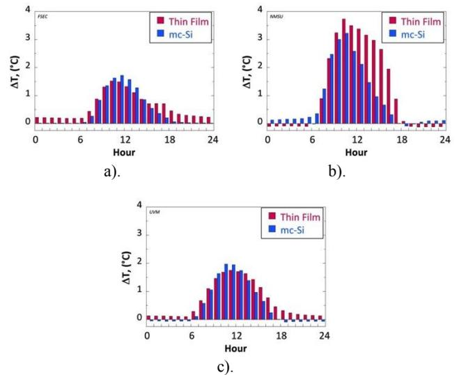
Fig. 8. Average Hourly Temperature Differences calculated for each technology for the full year. The mono-Si system at each location consistently operated at a lower temperature than the other two systems. The calculated  $\Delta T$  is the difference between each of the other technologies and the mono-Si system at their respective locations. FSEC a), NMSU b) and UVM c).
