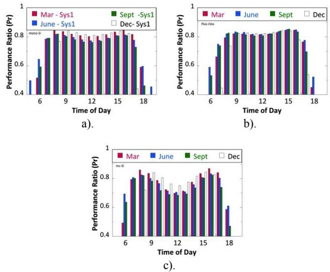
Fig. 7. Hourly Performance Ratio calculated for each technology for one month from each season. Mono-Si, a), Thin Film, b), and mc-Si, c). (Florida only).
