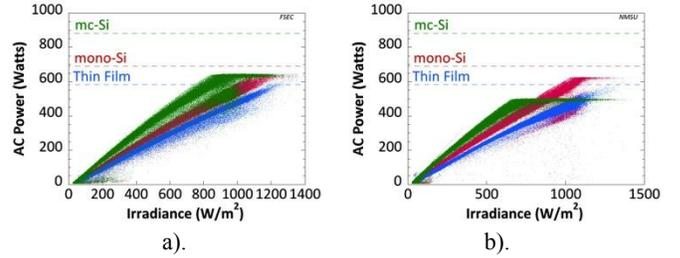
Fig. 3. Comparison of AC Power as a function of Irradiance for two sites. The inverters used for the mc-Si systems in both locations are undersized, leading to significant clipping. Clipping is also observed for the mono-Si system at high irradiance values.
