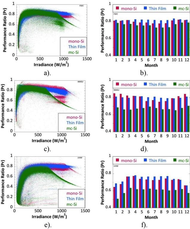
Fig. 6. Performance Ratio comparisons at FSEC, a) - b), NMSU, c) - d) and UVM, e) - f). Plots in on the left summarize instantaneous performance ratio as a function of irradiance and plots on the right show performance ratio calculated for each month.
