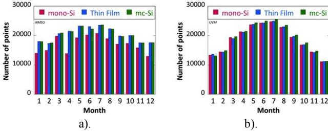
Fig. 2. Data filtering to remove noise resulted in an imbalance in the number of data points, a). NMSU and b). UVM. This negatively impacted comparisons of summed data such as total energy generation. Normalized quantities such as performance ratio were unaffected.
