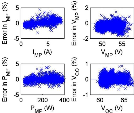
Fig. 2. Error in predicted voltage, current and power for model calibrated to outdoor data.
