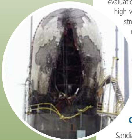
*Prestressed concrete containment vessel model structural failure mode testing.*
