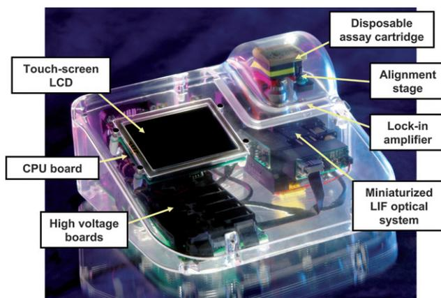
**Fig. 5** Prototype of the portable device for toxin diagnostics in a clear acrylic case showing internal components. The device is approximately 23 cm wide  $\times$  20 cm deep  $\times$  13 cm tall, and is powered by a conventional 12V–1A DC power adapter (not pictured).
