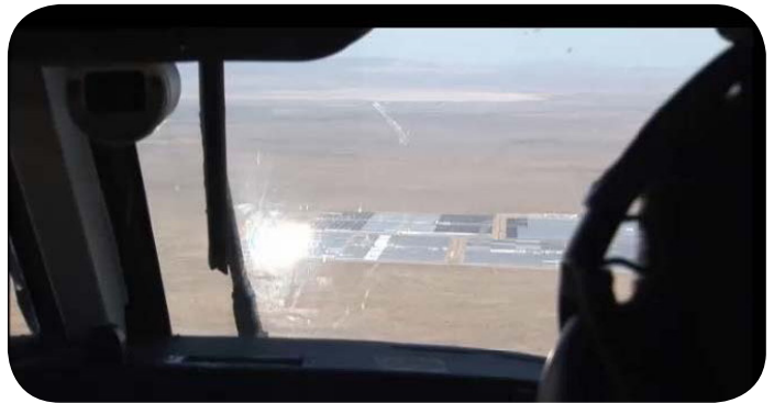
Glare from a large photovoltaic array, observed from C-12 cockpit at Kramer Junction, California (from Air Force Flight Test Center 412 TW at Edwards AFB, approval #13166).
