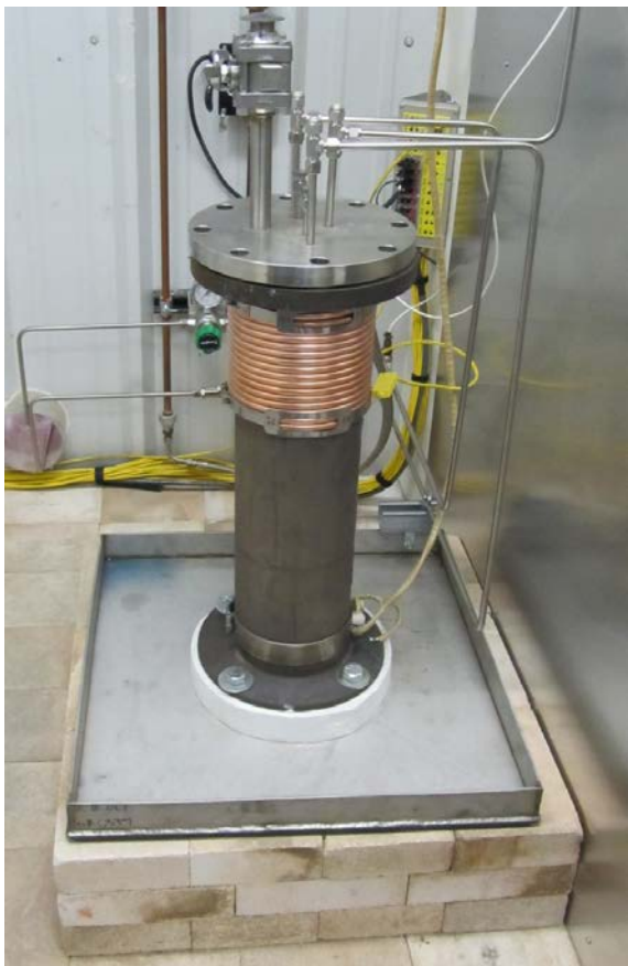
FIGURE 6. A MOLTEN SALT CORROSION TEST VESSEL SHOWN IN THE TEST CELL BEFORE INSULATING.
