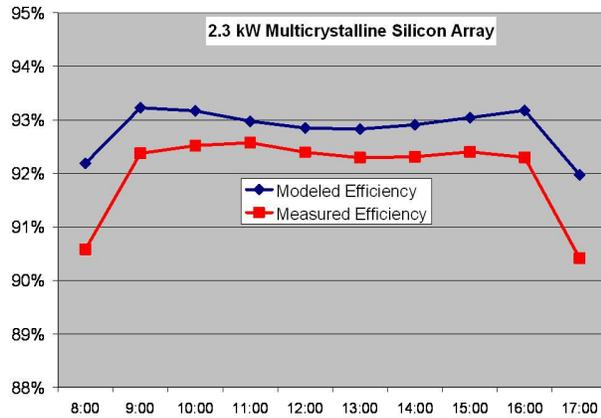
Fig 7. Comparison of Modeled vs. Measured Inverter Efficiency
