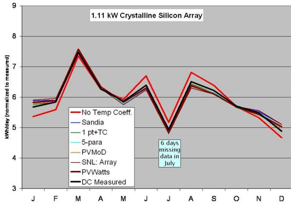
Fig 5. Normalized Modeled and Measured Array Output
