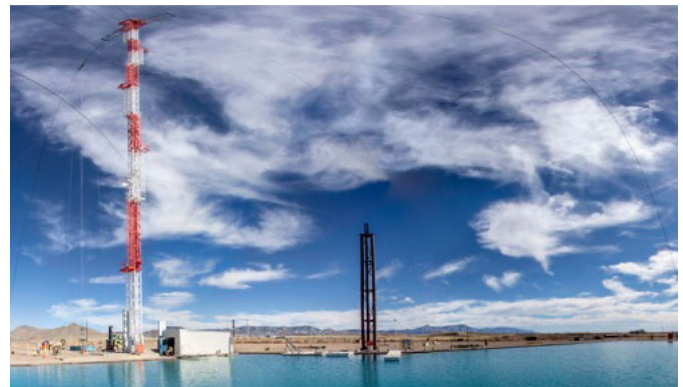
The Water Impact Facility, featuring a 300-foot drop tower and a large testing lake, provides a controlled environment for high-velocity water impact testing and underwater evaluations of marine technologies.
