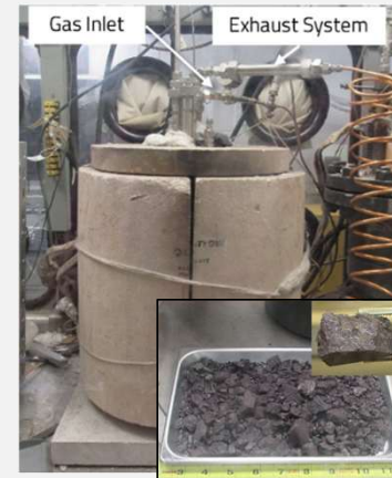
Engineering-scale UCl_3 salt production system (5 liters)
