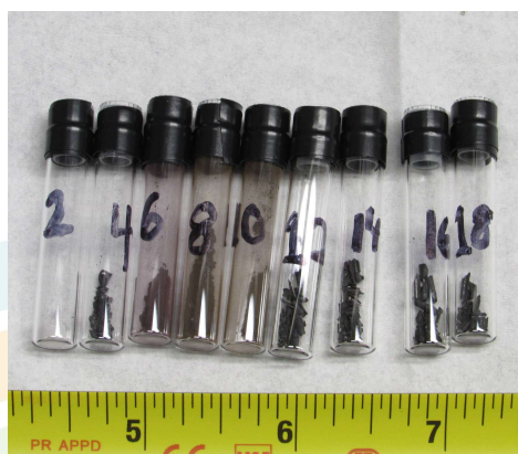
\text{UCl}_3 -NaCl-KCl LIBS vials sealed under argon
