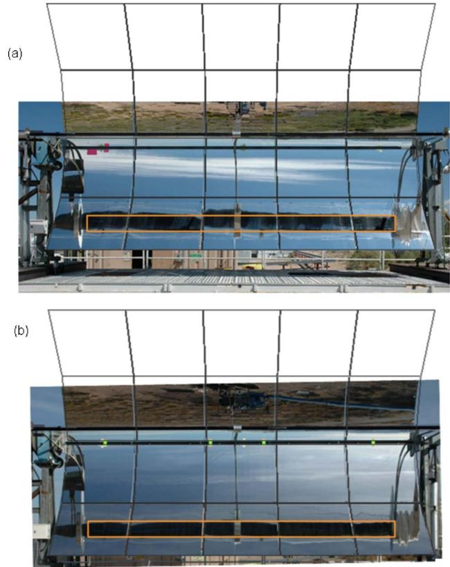
**Fig. 4** Theoretical overlay photograph of the LS-2 bottom outer row (a) before and (b) after TOP alignment. The TOP alignment called for more shims on the left side than the right side of the middle mirror to correct the slanted image.
