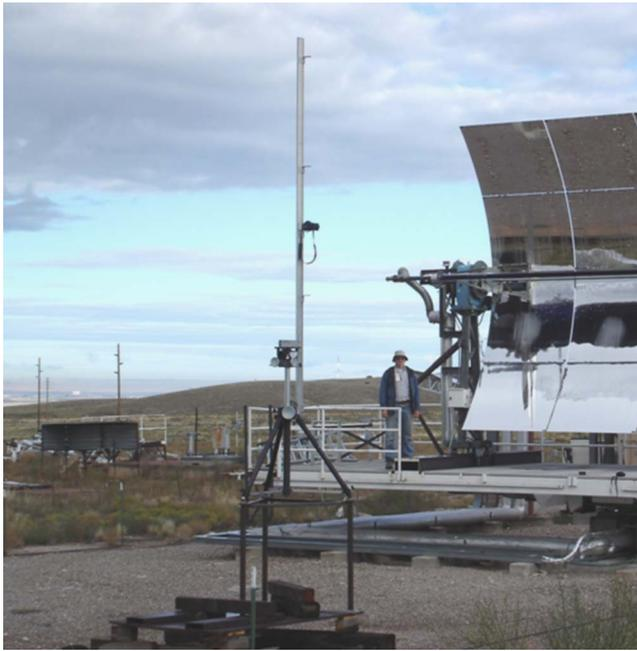
**Fig. 6** Photograph of the alignment fixture and LS-2 concentrator on the rotating platform at the NSTTF. The camera is mounted at the boresight position.
