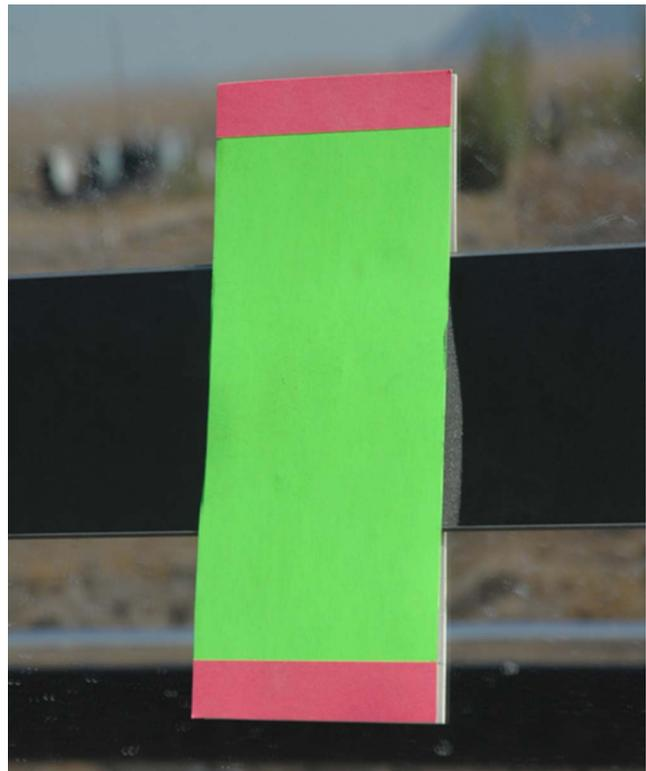
**Fig. 2 Photograph of a “boresight gauge” used to boresight the middle camera, HCE, and trough. A foam pad squeezes between the center two mirrors and accurately holds the color sight in position. The green center contrasts with the red edges and is 0.147 m long. The green center was sized to just be hidden from the camera by the HCE when on axis, but can be readily seen when off axis.**
