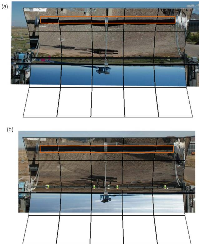
**Fig. 3** Theoretical overlay photograph of the LS-2 upper outer row (a) before and (b) after TOP alignment. Alignment is accomplished by adding shim washers on the side of the mirror in the direction the image needs to be moved.
