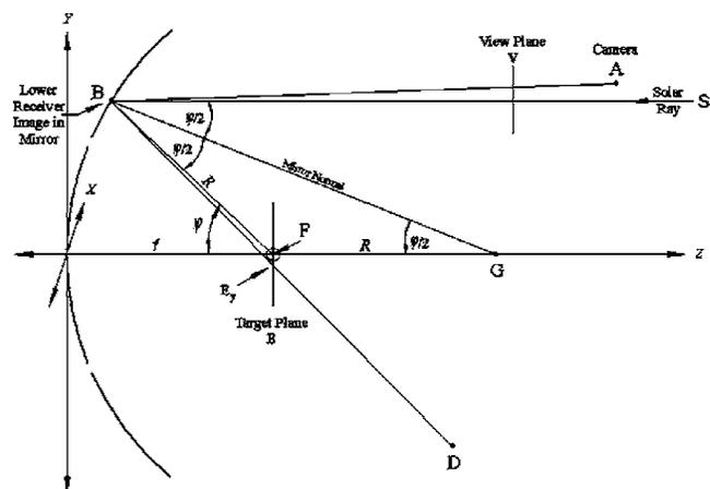
**Fig. 5** Schematic showing the coordinate system and locations of the mirror, HCE, target, focus, camera, and the solar rays for calculating the lower receiver edge position in the mirrors.
