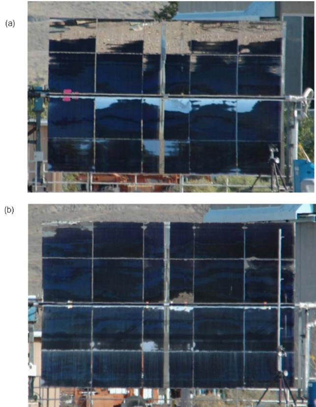
**Fig. 7** Distant observer photographs of the LS-2 module at the NSTTF (a) prior to and (b) after TOP alignment. Because the bottom mirror rows reflect the sky and the top mirror rows reflect the ground, misaligned regions appear blue on the bottom and brown on top. The distance from the camera to the trough vertex is approximately 460 m (1507 ft).
