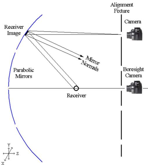
**Fig. 1 Schematic illustrating the TOP alignment technique. Accurately positioned cameras on an alignment fixture measure the position of the HCE image in the mirror. The boresight camera is used to align the fixture, HCE, and trough concentrator. The mirror is aligned to superimpose the HCE image onto the theoretically calculated image position.**
