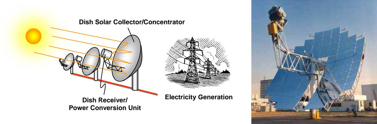
**Figure 6. Illustration and photo of dish/engine system**
