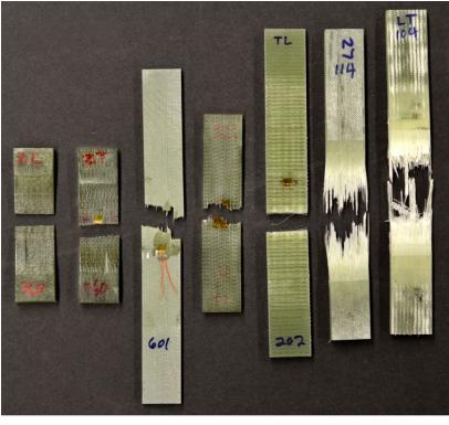
ZLT ZTL TZL TZL TLZ LZT LTZ tapered Figure 27a. Tensile Coupon Failure Photos
