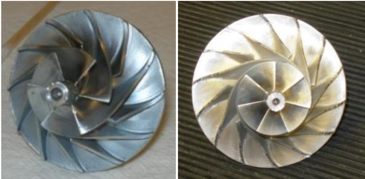
Figure 2-3. Main compressor (left) and recompressor (right) wheels.
