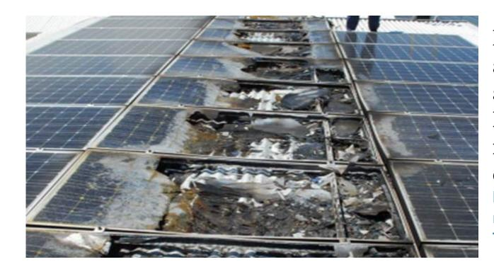
**Damage resulting from** an arc fault in the PV array. If left undetected, loss of life could result in addition to property damage. http://www.greentechmedia.co m/articles/read/Putting-Out
