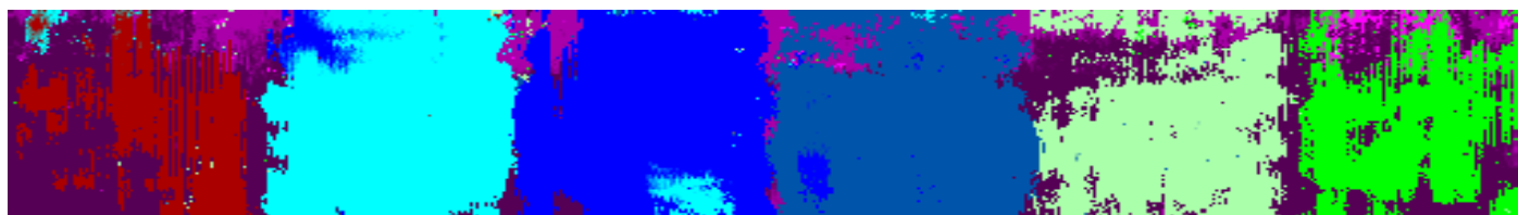
UT C-Scan Using Time of Flight
