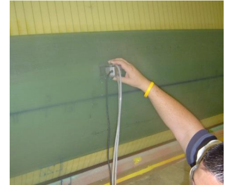
Phased Array Inspection
