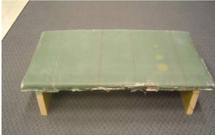
Shear Web/Spar with Disbands and Delaminations
