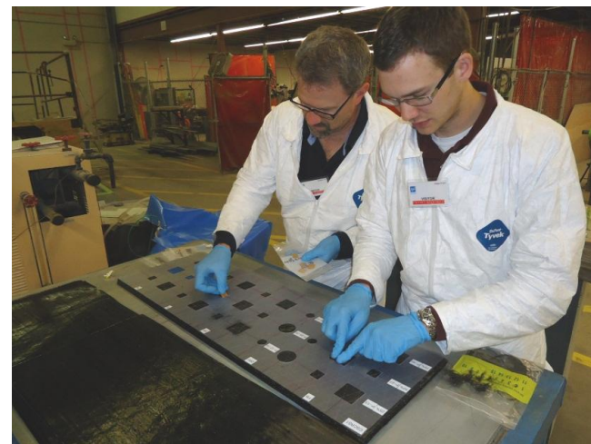
Flaws were placed at varying depths and locations using a template
