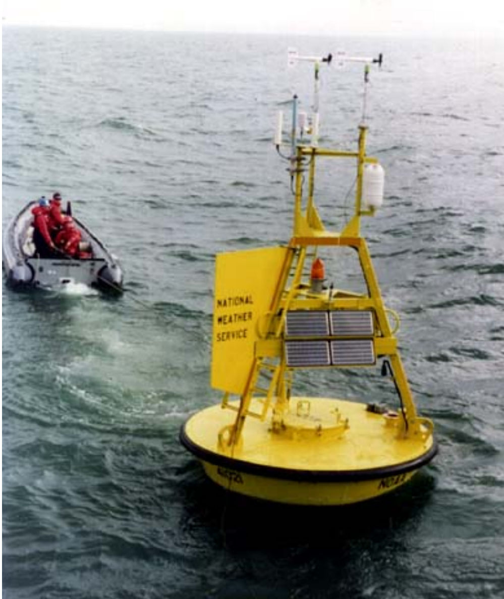
Figure 4.1: NDBC 3m “discus” buoy (image from http://www.ndbc.noaa.gov ).
