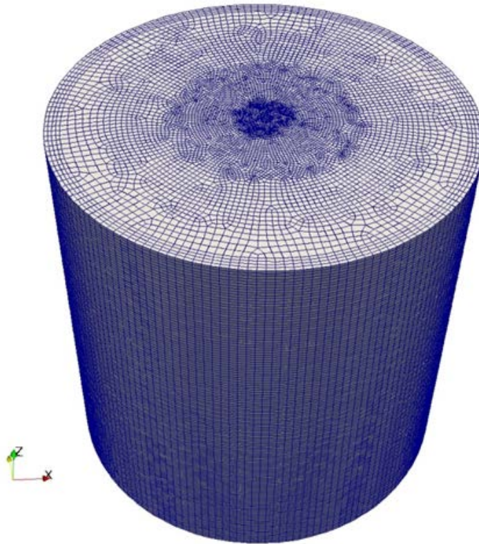
Figure 5-2 Mesh used for Gravitational Spill Simulation, Containing ~10 Million Elements.
