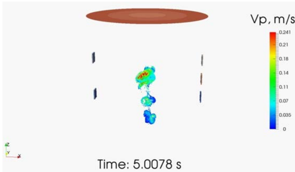
Figure 5-11 Fuego Results on Particle Velocity for 50 psig (0.34 MPa) Pressurized Release of TiO 2 at 5 seconds.
