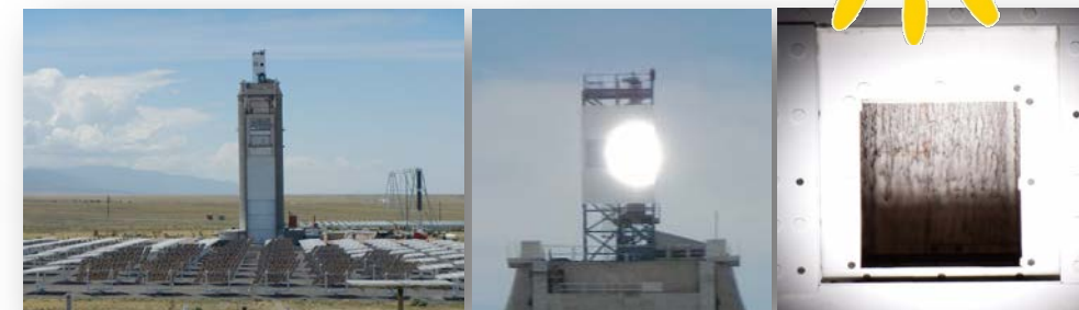
On-sun testing of the 1 MW t falling particle receiver at Sandia National Laboratories
