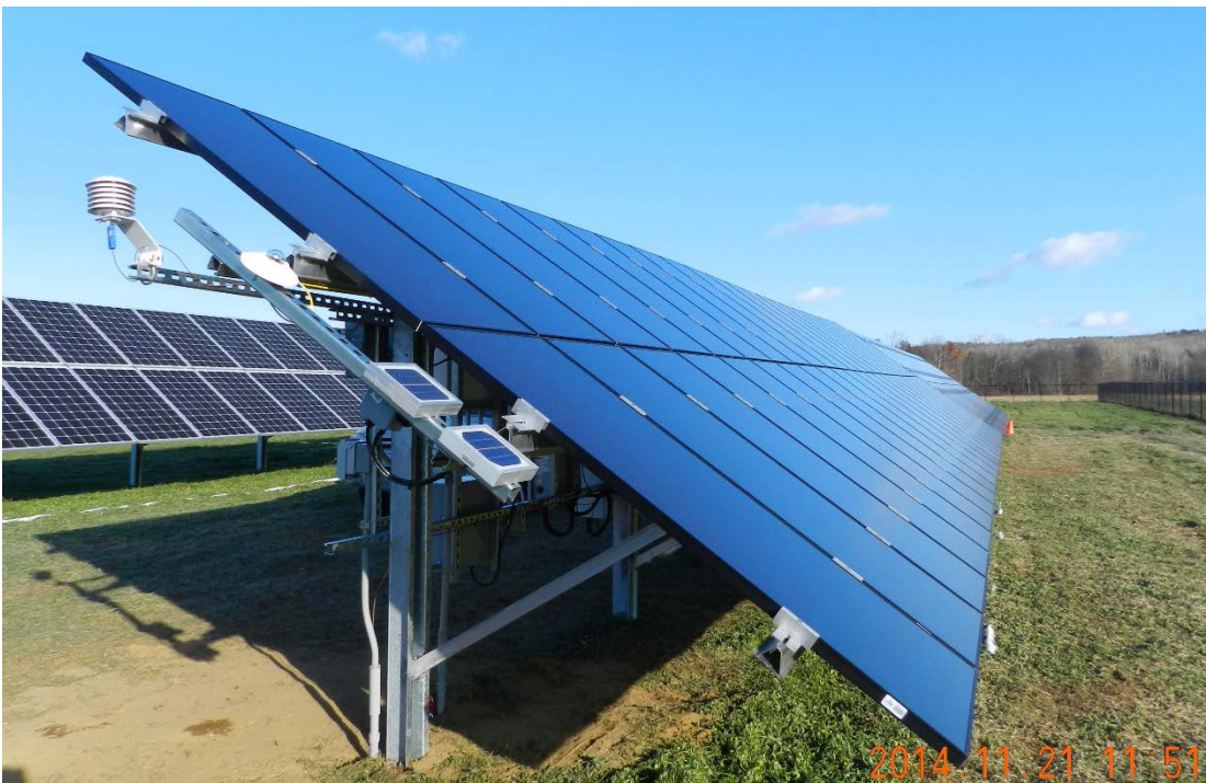
Figure 1: Photo of the meteorological instrumentation mounted on the west end of the Stion STO-140 array. Ambient temperature is measured by a shielded thermocouple (upper left); irradiance levels are measured by a plane-of-array pyranometer and two EETS reference cells, one of which is cleaned twice a week; the other is left to soil naturally.
