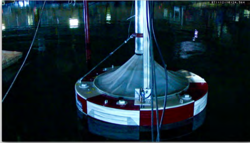
Figure 1.16: Pitch lock-out load cell installed on float.
