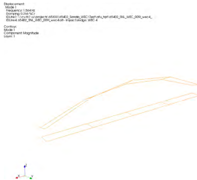
Figure 3-3. MASK bridge first vertical bending mode, carriage at west end.
