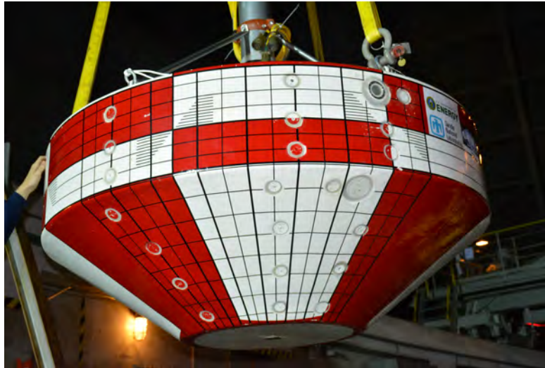
Figure 1.19: Pressure sensor ports on hull of device.
