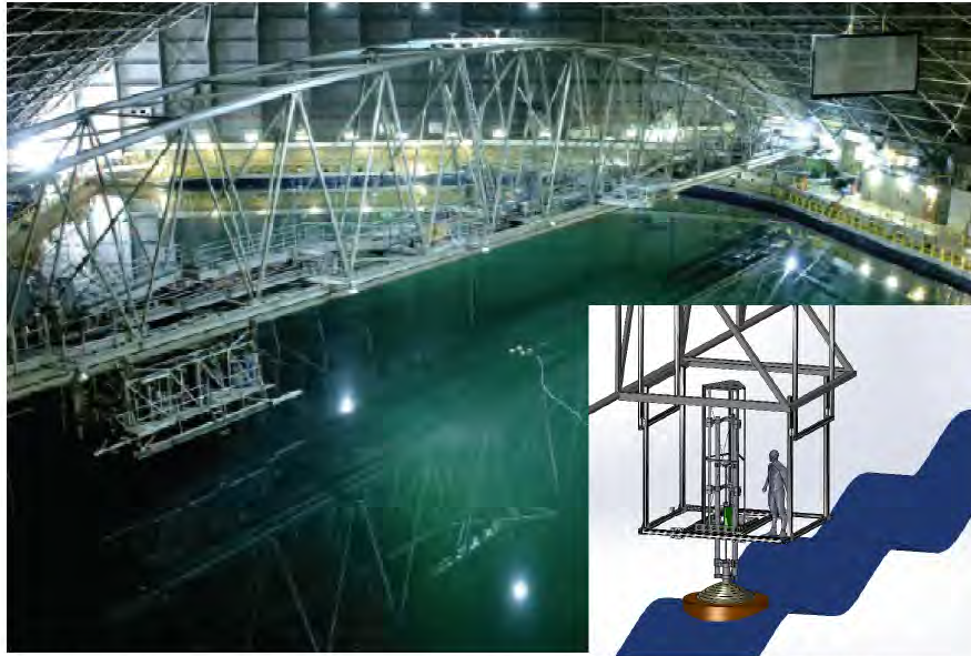
Figure 1-1. WEC system converts wave motion to electrical energy through a linear generator system.
