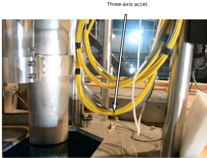
Figure 1.21: Location of triaxial accelerometer at base of PTO tower.
