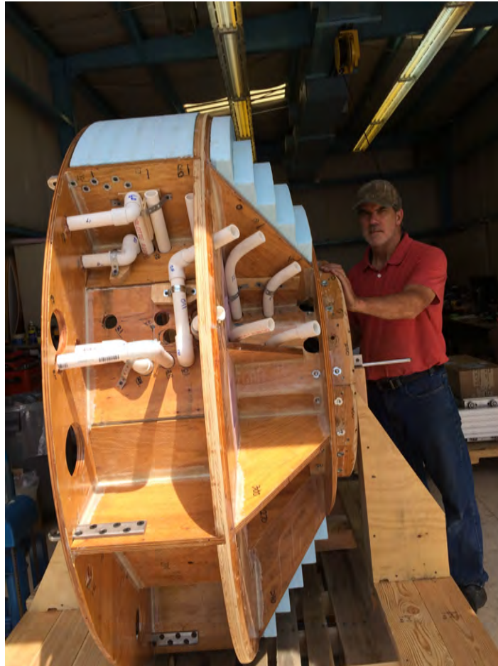
Figure 1.3: Photo during float construction showing internal plywood skeleton, foam and tubing for pressure sensors.
