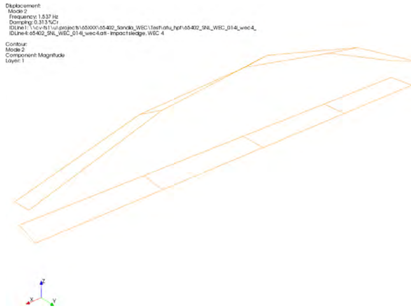
Figure 3-5. MASK bridge first vertical bending mode, carriage at mid-span.
