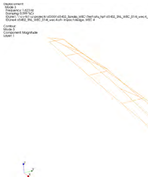
Figure 3-6. MASK bridge first torsion mode, carriage at mid-span.
