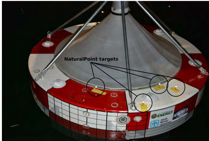
Figure 1.22: NaturalPoint optical tracking probes on float.
