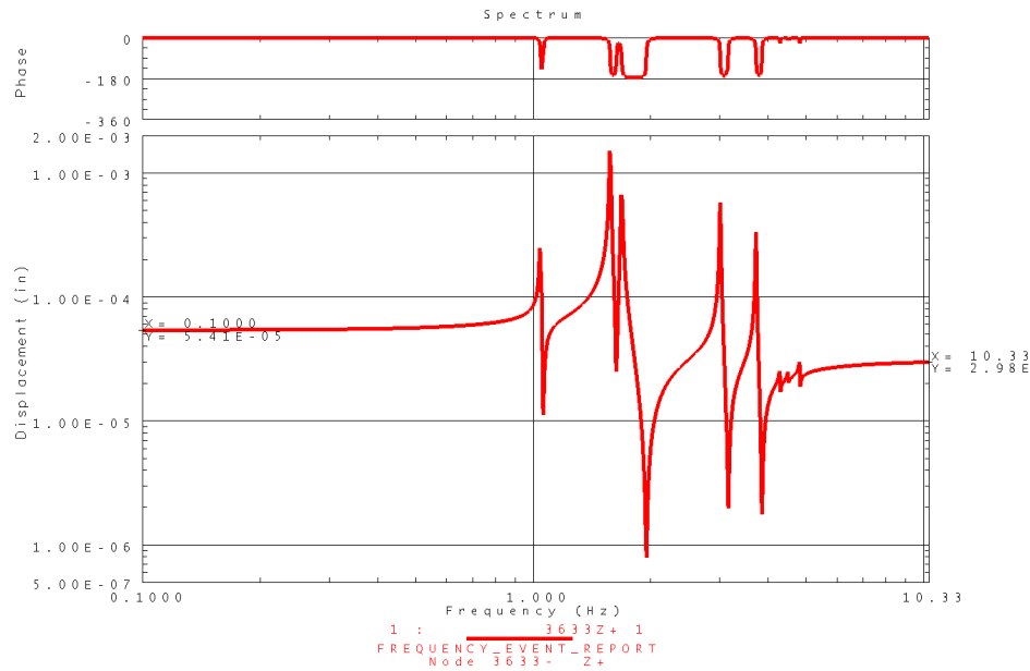
Figure 4-9. Driving point FRF for the WEC frame (based on a mode acceleration analysis).
