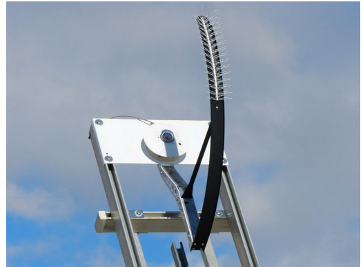
Fig. 1. Diffuse POA irradiance measurement for elevation-only rotations
