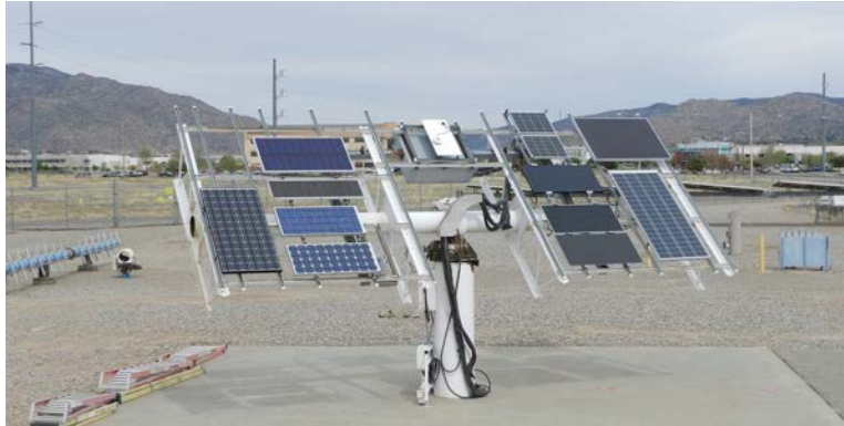
Figure 2. Modules under test on a two-axis tracker at Sandia
