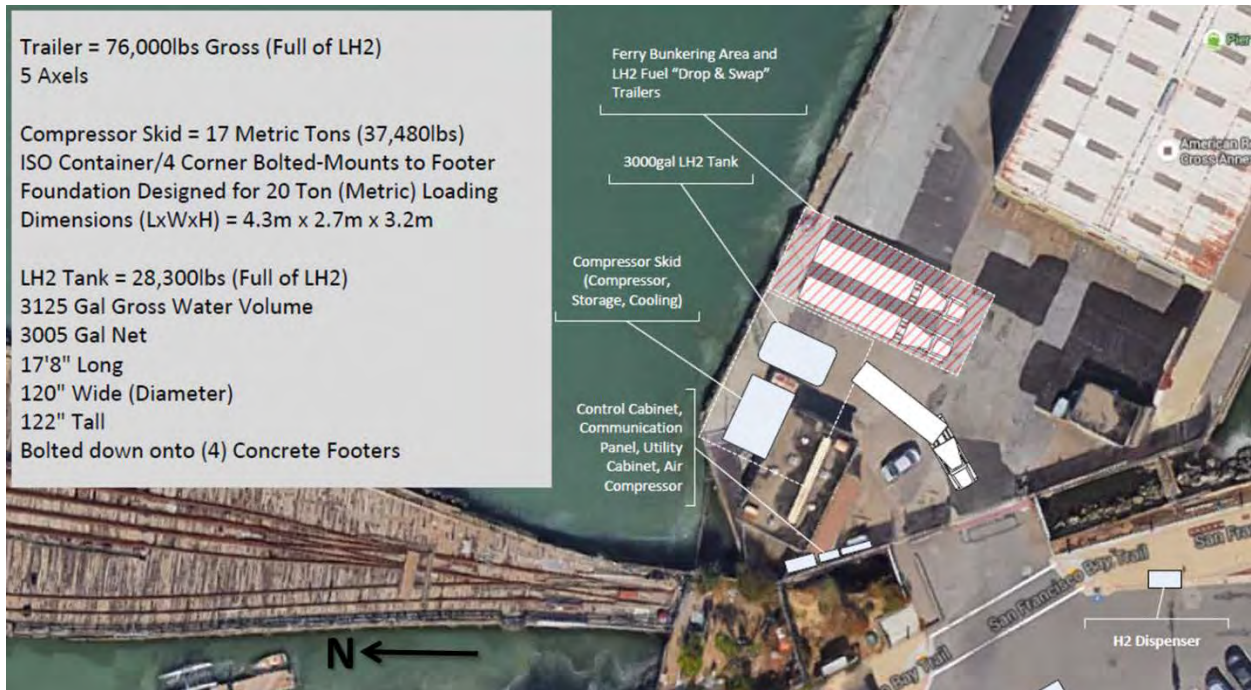
Figure 51: Example layout of hydrogen equipment at Pier 54's northwest berth supporting a vehicle fueling station and direct truck-to-vessel LH 2 bunkering. For orientation see inset on Figure 49. Layout courtesy of Linde.
