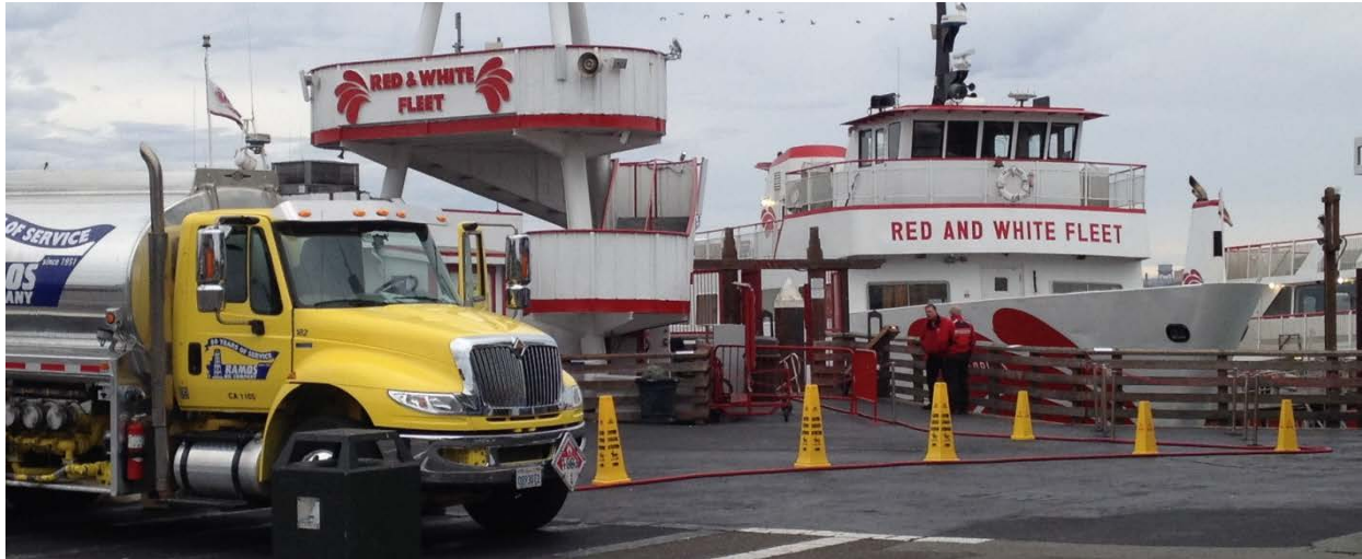
Figure 42: Conventional diesel fueling operation at the Red and White Fleet. The diesel truck (left) is transferring fuel through the red hose to the vessels in the background.
