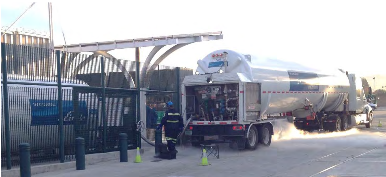
Figure 44: LH 2 transfer operation at AC Transit, Emeryville, CA, performed by Linde.
