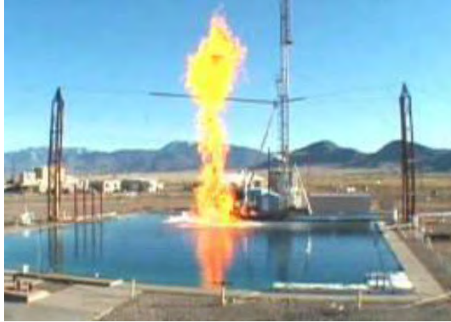
Figure 40: A 10-m diameter LNG pool fire from the Sandia Phoenix Tests. Figure reproduced from Reference [117].
