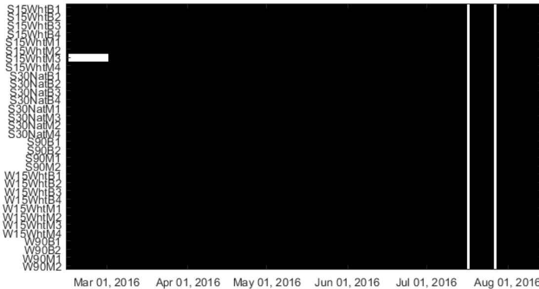
Figure 10: Data availability for all modules (y-axis) over the test period (x-axis). White areas shows missing data.
