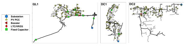
Figure 3. Topologies of the full circuit models of feeder QL1 (left), DC1 (middle), and DC2 (right)
