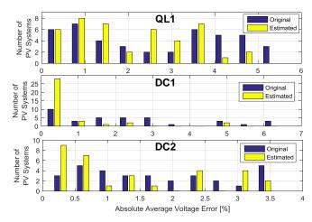
Figure 5. Feeder QL1 (top), DC1 (middle), and DC2 (bottom) absolute average voltage error for each PV system simulated with the original (in blue) and estimated (in yellow) parameters
