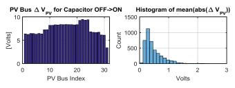
Figure 4. Feeder DC2 capacitor state impact on the PV voltages
