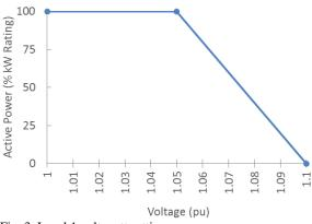
Fig. 3. Level 1 volt-watt setting.
