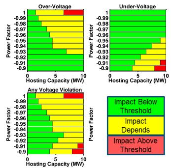
Fig. 1. Hosting capacity analysis for feeder 631 at various inductive power factors.
