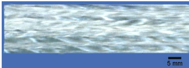
Figure 13. Aligned strand structure
