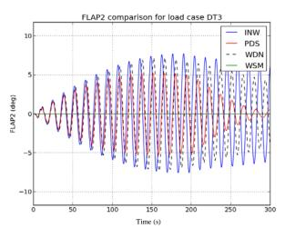
Figure 12. Comparison of Flap 2 pitch motion for load case DT3.
