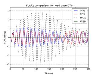
Figure 16. Comparison of Flap 2 pitch motion for load case DT6.
