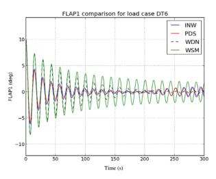
Figure 15. Comparison of Flap 1 pitch motion for load case DT6.
