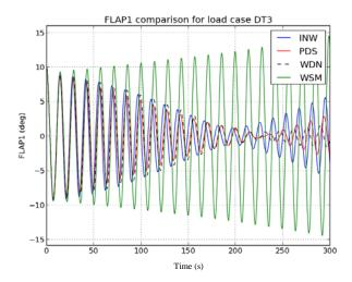
Figure 11. Comparison of Flap 1 pitch motion for load case DT3.
