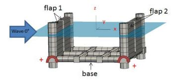
Figure 2. Schematic of the F3OF inspired by the Langlee device
