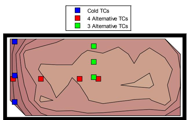
Fig. 7. Alternative thermocouple configurations.
