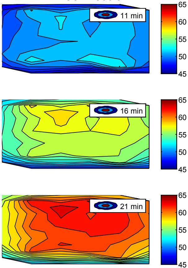
Fig. 5. Temperature maps for the 72 cell module.
