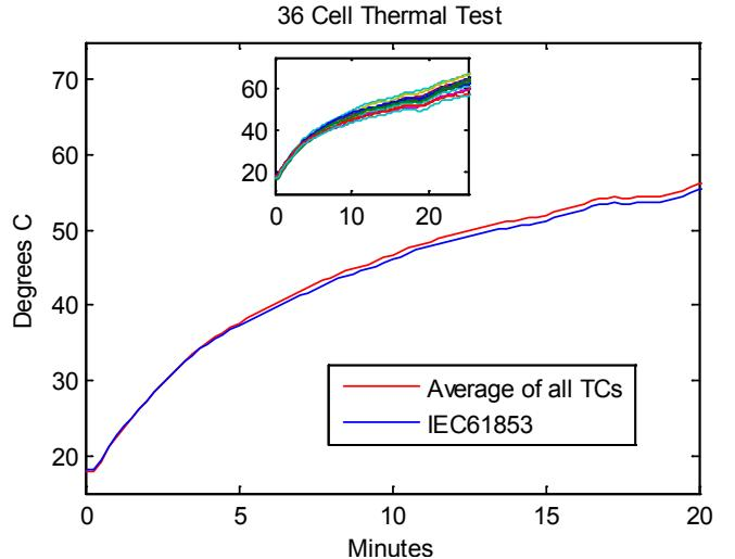
Fig. 4. Temperature measurements for the 36 cell module.
