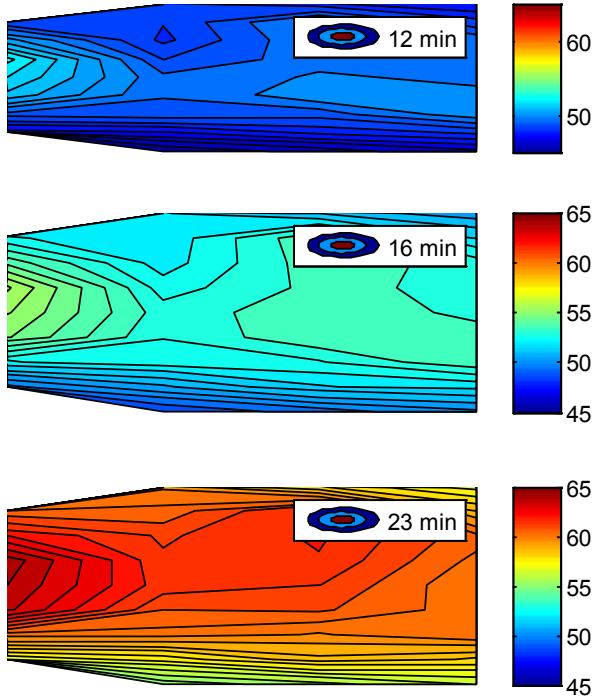
Fig. 6. Temperature maps for the 36 cell module.
