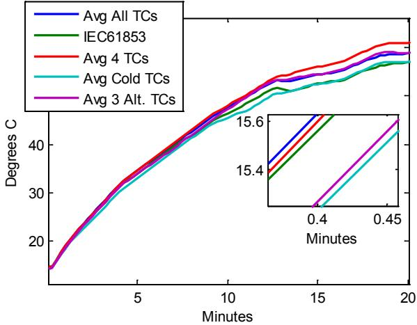
Fig. 8. Average temperatures for various combinations of thermocouples.
