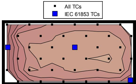
Fig. 2. Thermocouple locations on the 72 cell module.
