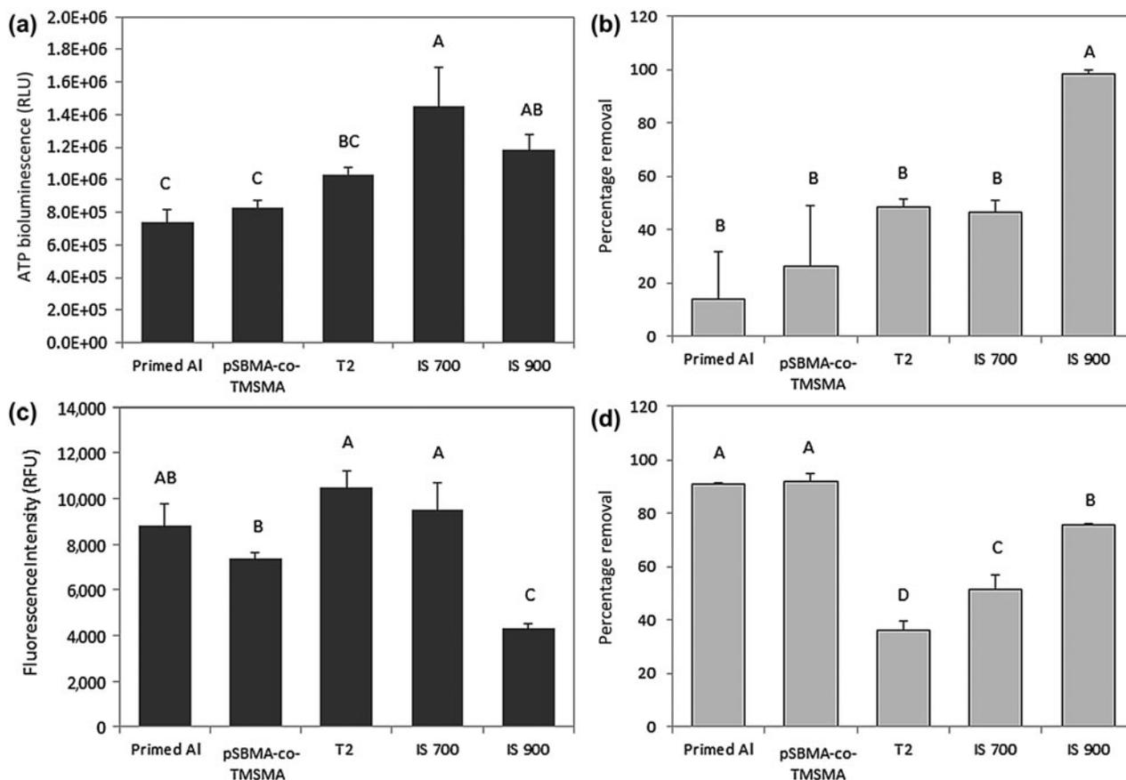
Figure 5. Evaluation of *C. lytica* biofilm (a) retention and (b) removal and *N. incerta* cell (c) attachment and (d) removal on pSBMA-co-TMSMA and control coatings. Data points that share a letter are not statistically different from one another (ANOVA,  $\alpha = 0.05$ ).
