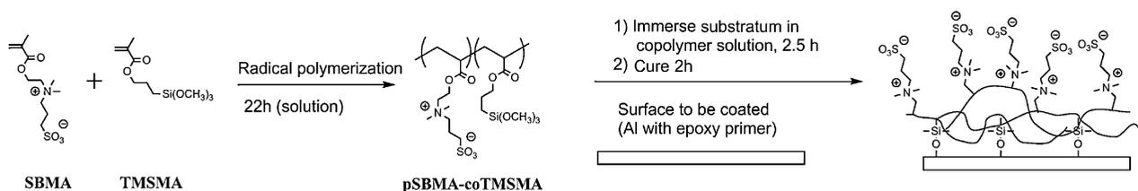
Figure 4. Synthesis and application of the pSBMA-co-TMSMA coating.
