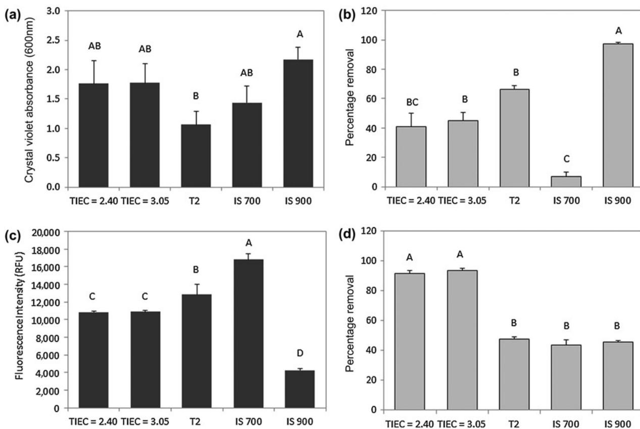
Figure 3. Evaluation of *C. lytica* biofilm (a) retention and (b) removal; and *N. incerta* cell (c) attachment and (d) removal on ZTMPS and control coatings. Data points that share a letter are not statistically different from one another (ANOVA,  $\alpha = 0.05$ ).
