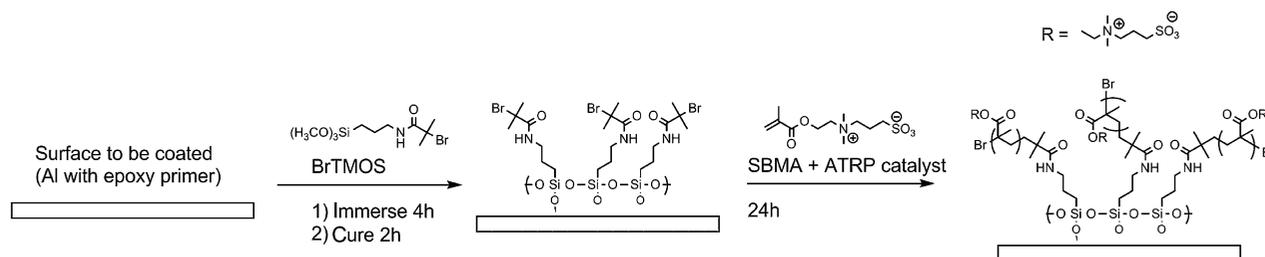
Figure 6. Synthesis and application of the gpSBMA coating.
