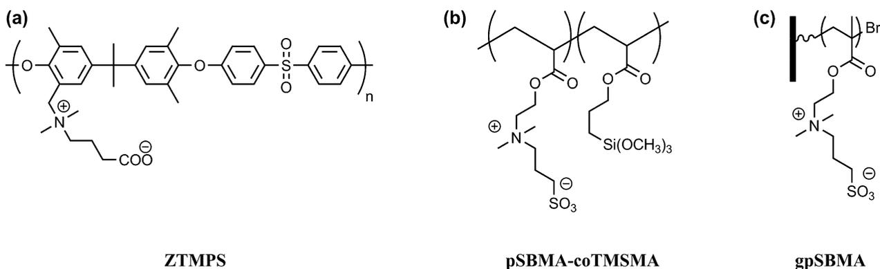
Figure 1. Structures of the zwitterionic coatings synthesized for this study.
