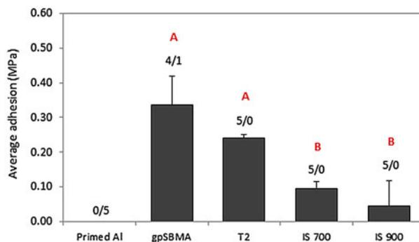
Figure 8. Average adhesion values for reattached adult barnacles that were dislodged from the coating surfaces without incurring visible damage or breakage to baseplates. The ratios above each bar indicate the total number of barnacles removed without baseplate damage vs the number of barnacles that exhibited baseplate damage during force gage removal. Data points that share a letter are not statistically different from one another (ANOVA,  $\alpha = 0.05$ ).
