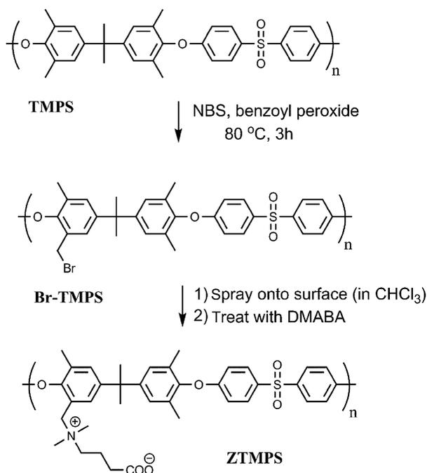
Figure 2. Synthesis and application of ZTMPS coatings.
