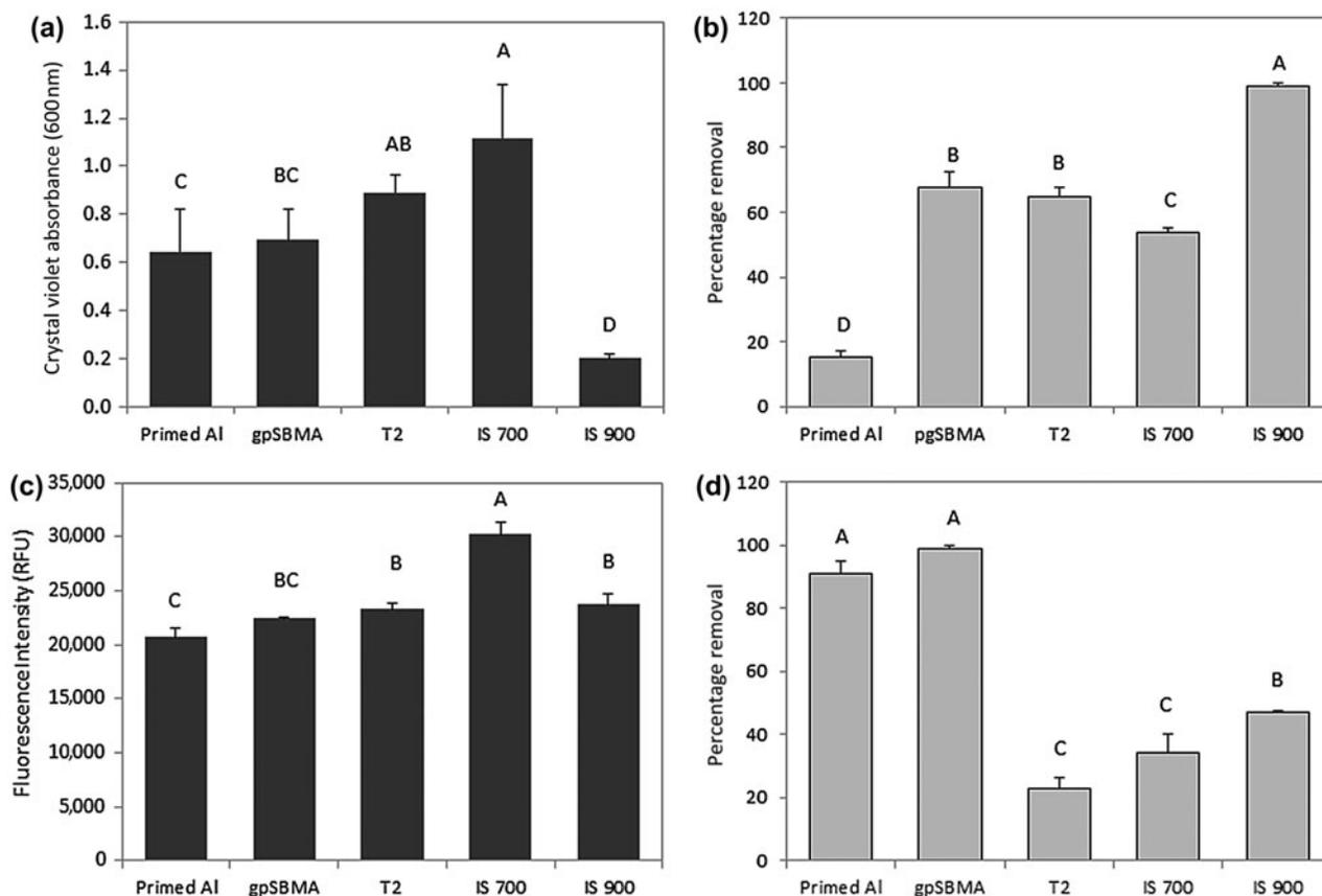
Figure 7. Evaluation of *C. lytica* biofilm (a) retention and (b) removal and *N. incerta* cell (c) attachment and (d) removal on gpSBMA and control coatings. Data points that share a letter are not statistically different from one another (ANOVA,  $\alpha = 0.05$ ).
