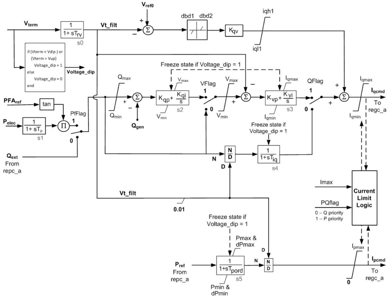
Figure 3. Renewable energy electrical control module for PV plants.
