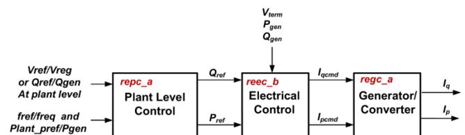
Figure 1. Central station PV plant model interconnection diagram.
