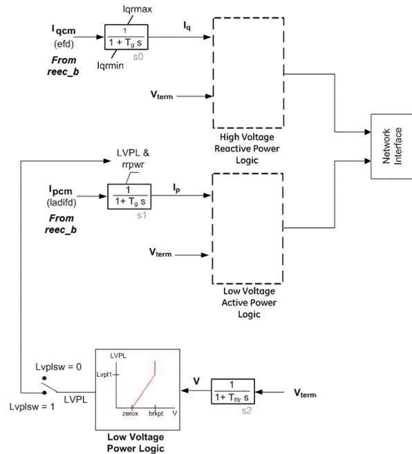
Figure 2. Renewable energy generator/converter module.
