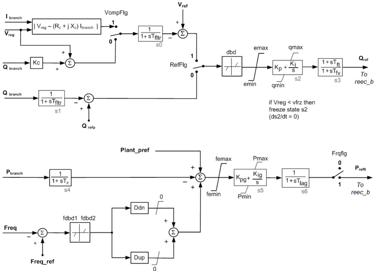
Figure 4. Renewable energy plant-level control module.
