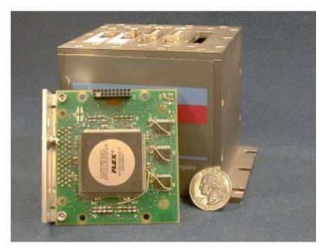
Figure 2-10. The Programmable Accurate Time Synchronization Module
