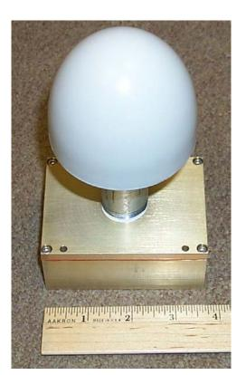
Figure 2-11. GPS Receiver/Antenna Configuration.
