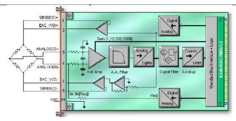
Figure 2-8. Full-bridge Strain Gauge Schematic.
