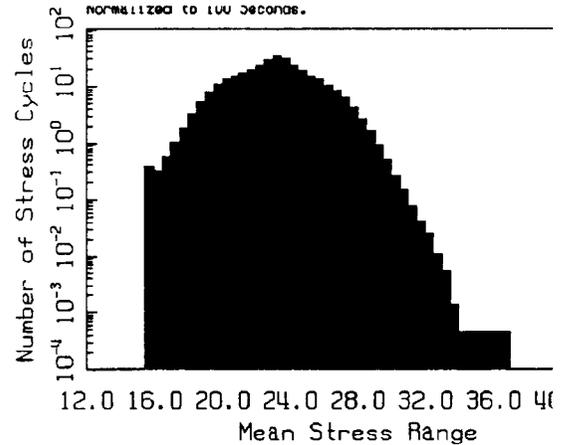
**Figure 9. Mean Stress Cycle Count Distribution for Synthesized Time Series Data at Positive 45 Degrees.**
