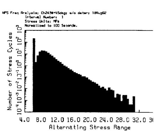
**Figure 8. Alternating Stress Cycle Count Distribution for Synthesized Time Series Data at Positive 45 Degrees.**
