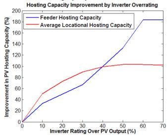
Figure 6. Feeder 1 overall (blue) and locational (red) hosting capacity improvement as a function of PV system inverter oversizing when using Volt-Var control.
