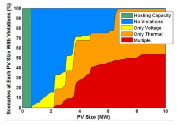
Figure 2. Base case (no inverter control) hosting capacity profile for Feeder 1.
