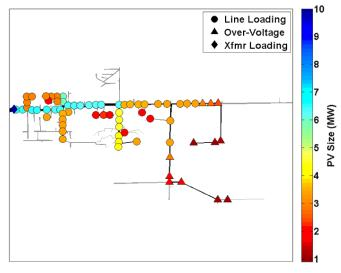
Figure 5. Feeder 1 locational hosting capacity with Volt-Var control on the PV inverter.
