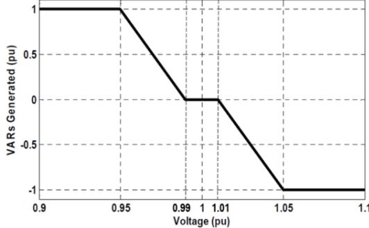
Figure 1. Volt-Var droop control curve used for PV system inverters in this research.
