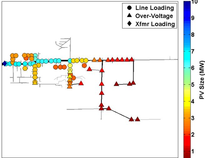
Figure 4. Feeder 1 base case locational hosting capacity.
